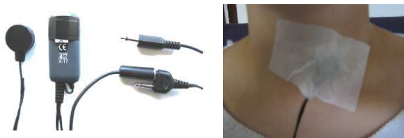
Fig. 1 Commercial larynx microphone (left); positioning of the microphone next to the larynx of the patient (right)
